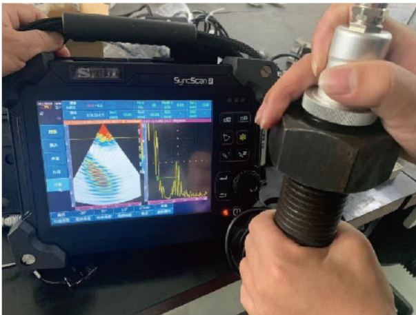
PA Inspection for Bolt
