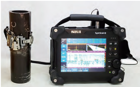
PAUT solution for small pipe weld
