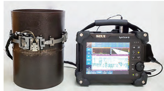
PAUT solution for medium pipe weld
