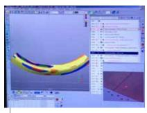
The color-coded areas graphically illustrate the geometric deviation of the leading edge surface.
