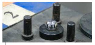
Detail of tooling ball on rotating table
