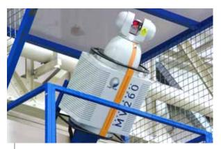
Airbus opted for an automated Laser Radar inspection cell that drastically speeds up nose cowl inspection.
