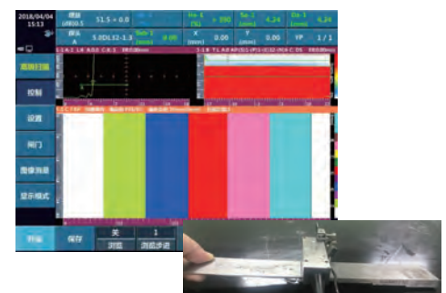
Wall thickness of the thin-walled step test block is displayed in different colors
